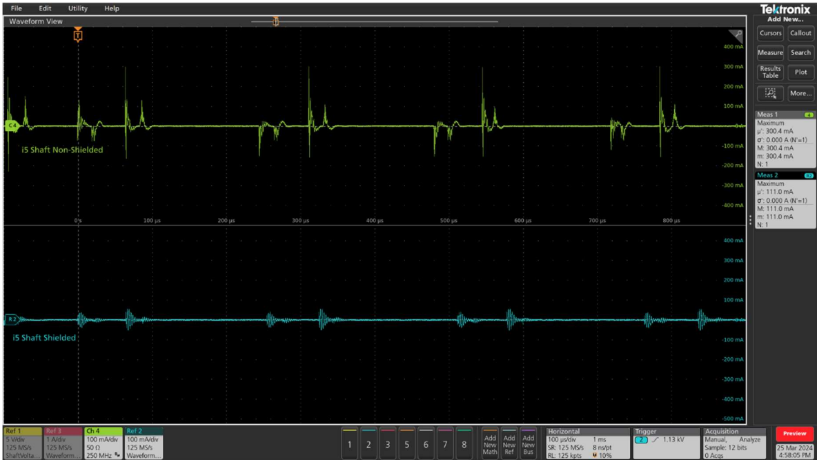
Figure 2: Motor Shaft Current Measurements of Properly Installed VFD Cable vs. Standard Cable
