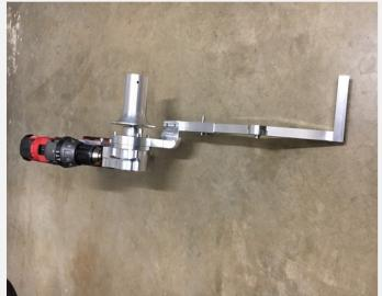
Puller handle is designed for ergonomic convenience and tool control.
