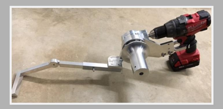
The CP1000 measures only 24" long when fully extended. When collapsed it easily fits into a tool bag. The heavy-duty drill chuck and handle lock attachment provide a sturdy base of operation. Wires up to 1/0 gauge can be pulled using the device.
