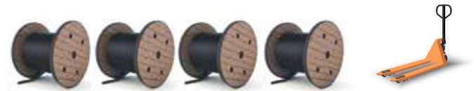
Feeders: The Traditional Way 4 Reels, 1 pallet jack, 4 reel jack stands, 4 axles, 6 electricians
