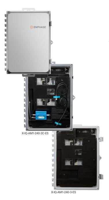
The IQ Combiner 3-ES/3C-ES with IQ Gateway and integrated LTE-M1 cell modem (included only with IQ Combiner 3C-ES) consolidates interconnection equipment into a single enclosure and streamlines PV and storage installations by providing a consistent, pre-wired solution for residential applications. It offers up to four two-pole input circuits and Eaton BR series busbar assembly.
