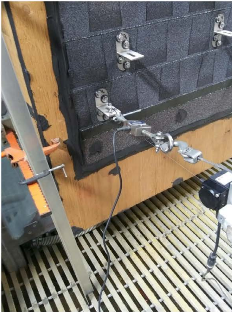
Photo No. 1 Pullout Test
